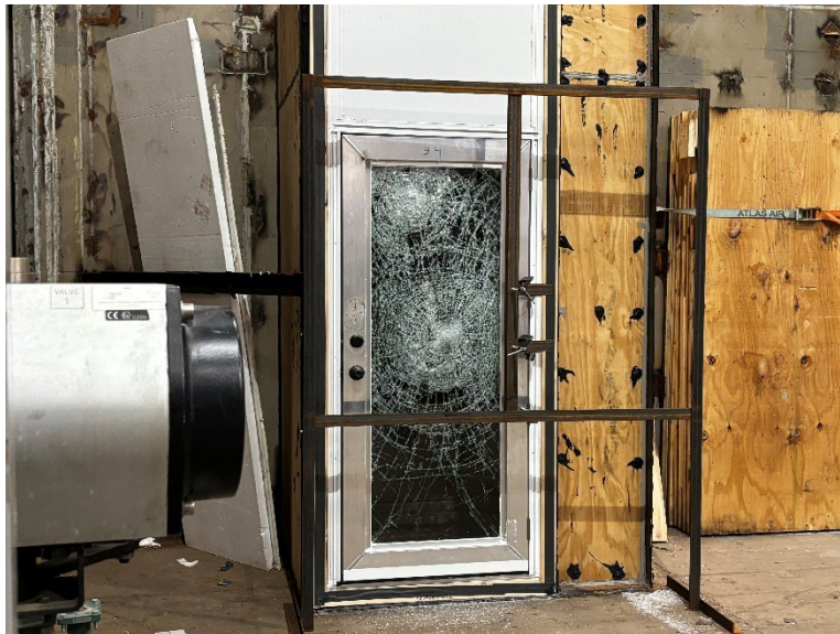
Photo No. 16 TAS 203 Test Setup
